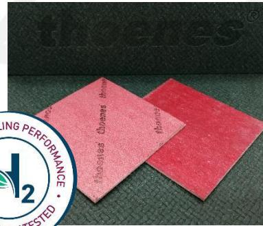
The gasket material sheet has been specially developed for demanding applications where only low bolt loads permissible and flange irregularities need to be compensated. It offers a high compressibility and an increased recovery in addition to improved mechanical and thermal performances. It can be used for sealing mineral oils, fuels, lubricants refrigerants, steam, air and many other media.
